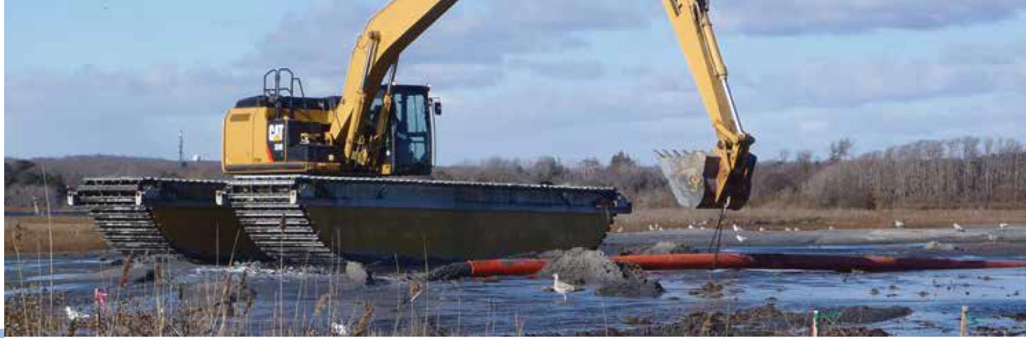
Amphibious excavator moving dredge slurry pipe © Save the Bay
